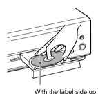
"TOC" starts to flash. The recorder starts to read the TOC (Table of Contents) data and shows the type of the disc in the deck on the front panel display.
