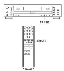
1 Press ERASE one time (for a finalized disc) or twice (for unfinalized disc) until "DISC ERASE" appears in the front panel display.
